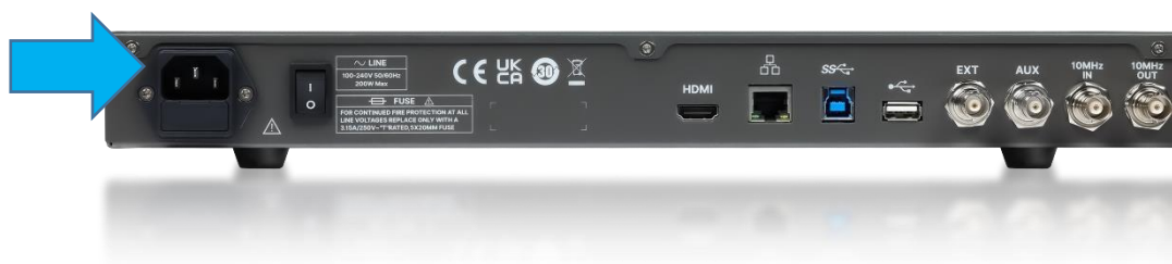
Figure 2 SDS5000L connect the power cord
